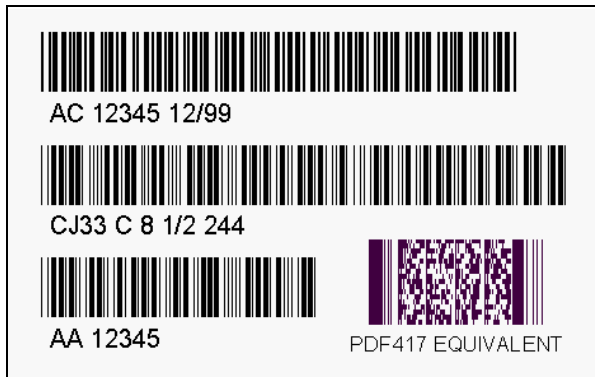
Figure 4 – Actual Wheel Barcode Label Comparing Code 39 and PDF417
